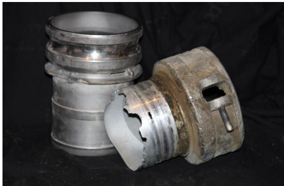
Above Photo: Unlined Kamlocks after several weeks of service in frac sand application.
